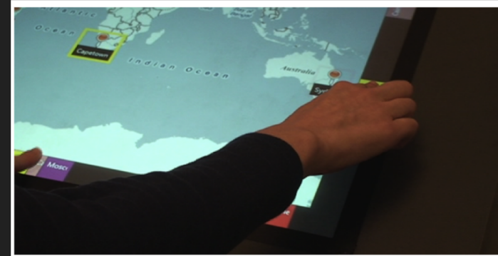
Figure 1. Access overlays allow a blind user to accurately locate items on a 2-D touch screen map.
