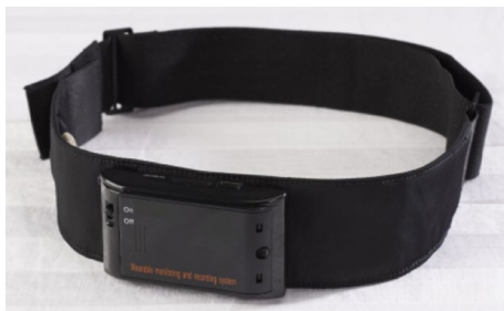
Fig. 1 Our waist-belt HRV monitoring system
